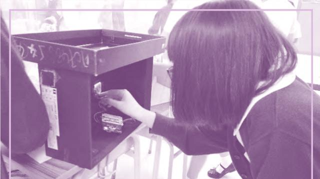
Using a shoebox as a medium, a microbit chip with a built-in microphone sensor is put inside to detect how effective the headphone is in noise cancellation.
